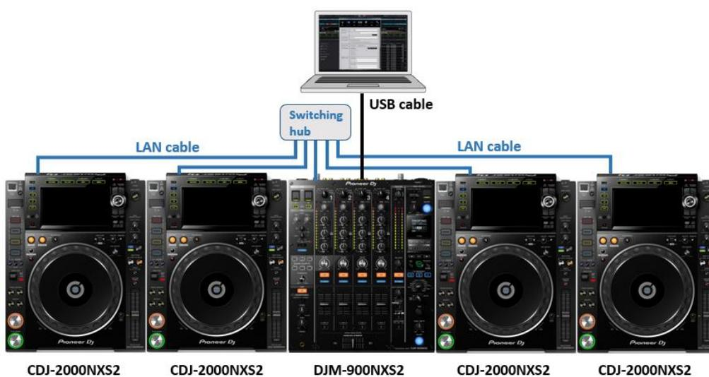
This section describes how to set up connection with DJM as an audio interface using an example of connection with DJM-900NXS. Install driver software before connection as described in *1.2.2 Driver installation*.
